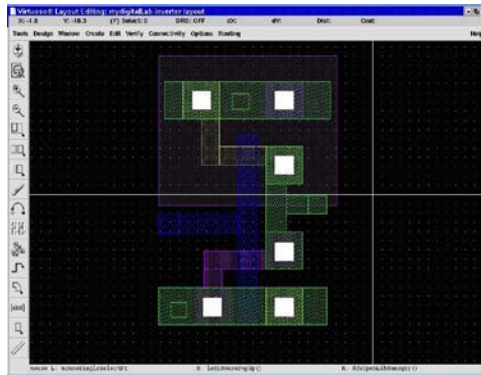
Figure 2: Layout of a CMOS inverter gate.
